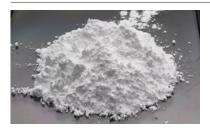
**PROPOLDER™** is polypropylene fine powder. **PROPOLDER™** has two kinds of base resin and various particle size ranges for special applications.
